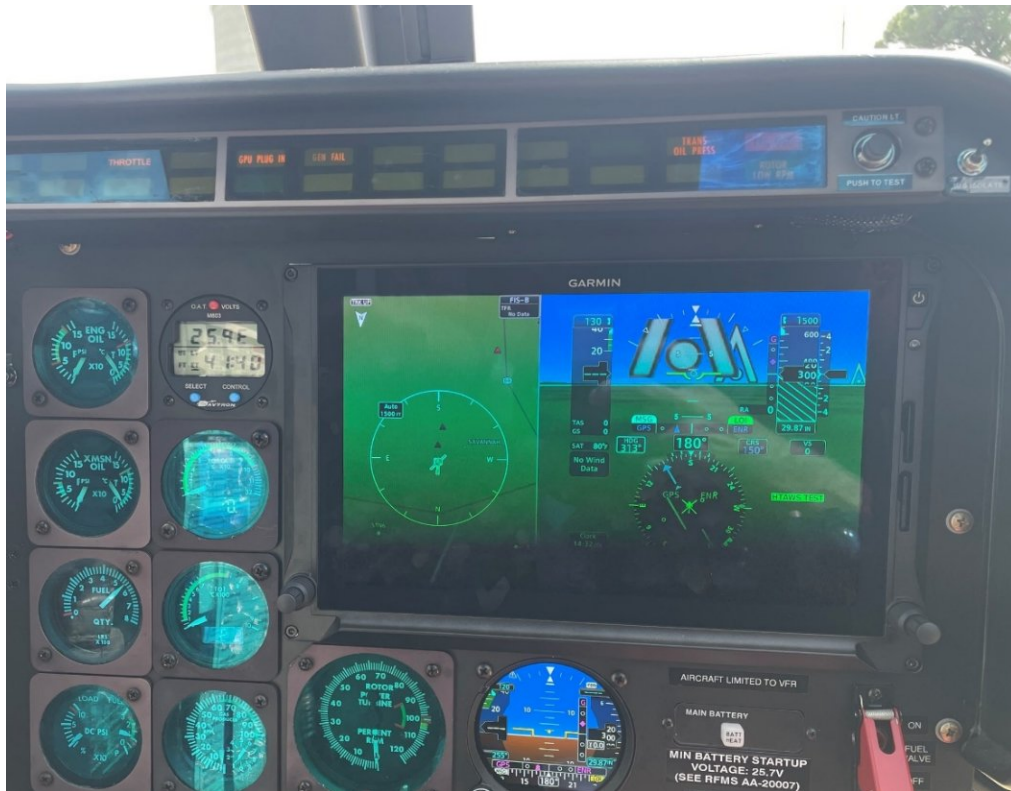
Figure 2 - Exemplar of instrument panel as configured in accident helicopter.
